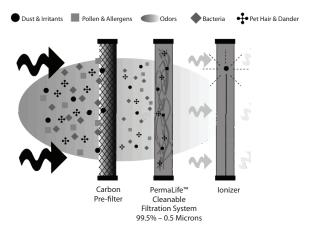
Fig. 1 - Illustration of the Air Filtration System
